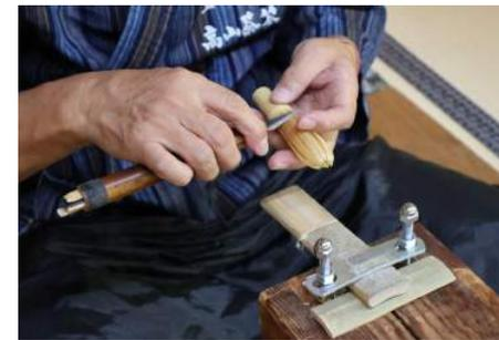
To strengthen the fibers inside, it is necessary to first age the bamboo used for the tea whisks for 3 years. The aged bamboo is cut in the cold winter months from December to January to remove oils, then boiled in an iron pot. After that, it is dried outdoors for 2 months and, once it turns white, put in storage for an additional 2-3 years. I was surprised by how long it takes just to prepare for tea whisk creation.
