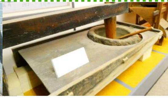
*Karausu* (or large mortar and pestles) are a tool used in the traditional making of mochi (rice cakes). They are operated with 2 people, with one person on the left side holding down the pedal with their foot using all their strength to raise the wooden mallet, and the other on the right side shaping the mochi with the pestle while the mallet is raised. When the first person steps off the pedal, the wooden mallet falls down, pounding the mochi.
